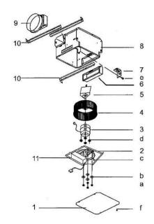
Replacement installation: Remove the screw (part c), then take out the motor plate (part 2) from the housing (part 8) by pushing down the rib in the plate while pulling out on the side of the housing. Replace the broken parts.
