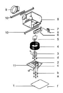
Replacement installation: Remove the screw (part c), then take out the motor plate (part 2) from the housing (part 8) by pushing down the rib in the plate while pulling out on the side of the housing. Replace the broken parts.
