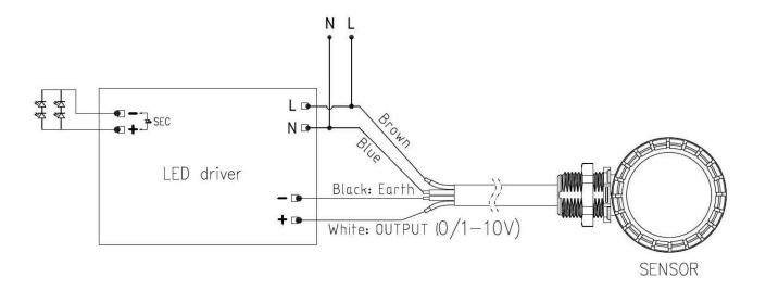
\*The sensor is designed for connect one load only.
