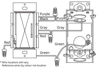
Dimming with ON / OFF Control Wallbox Wiring
