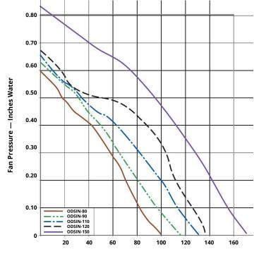
Fan Flow Rate CFM Standard Air
