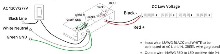
Output wire 14AWG RED to LED positive side (+), BLACK to LED negative side (-)
