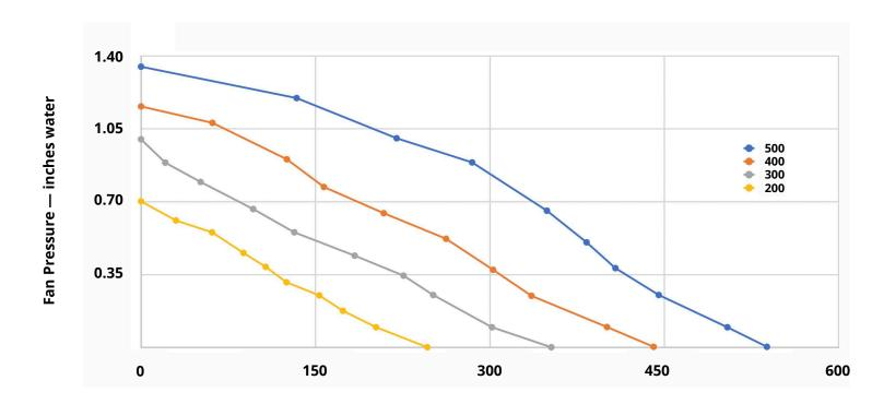
Fan Flow Rate — CFM Standard Air
