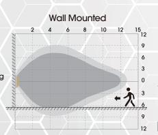
This figure indicates the maximum distance at the highest mounting height with 100% sensitivity.
