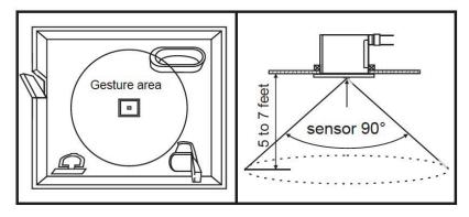
**For ODD-100HS+MS**, turn ON the switch to activate sensor and continuous ventilation system. The fan will run continuously at the pre-set low speed. When motion is detected, the fan speed increases to high speed. When the person exits the area, the fan remains working at high speed until the delay time has passed (adjustable 20 minutes). After the time delay, the fan speed is reduced to the continuous ventilation rate.
