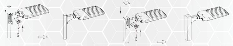
STEP 8: Loosen the locking bott by a wrench to adjust the fixture to a appropriate angle, adjustment range 15°, then tighten this locking bott.
