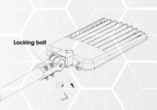
**STEP 7:** Loosen the locking bolt in the SB-SLIP FITTER by a wrench to adjust fixture to a appropriate angle, adjustable angle range 90 then this locking bolt.
