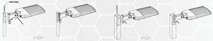
ATTENTION: When install to round pole, please remove the rubber gasket.
