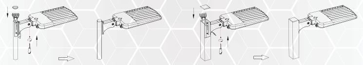
STEP 7: (ii) Push the connected wires into bracket junction box, close the box cover by tightening the screws, then close the pole's top cover.
