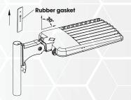
**STEP 5:** Pass the fixture's AC input wires through the pole, pull them out together through the pole for wire connection, Or pass the pole-wires into SB-POLE-M2 bracket, pull them out together with fixture's AC wire from junction box, connect the fixture's AC input wires to pole-wires with connectors, L to L (black), N to N (white), PE to PE (green).
