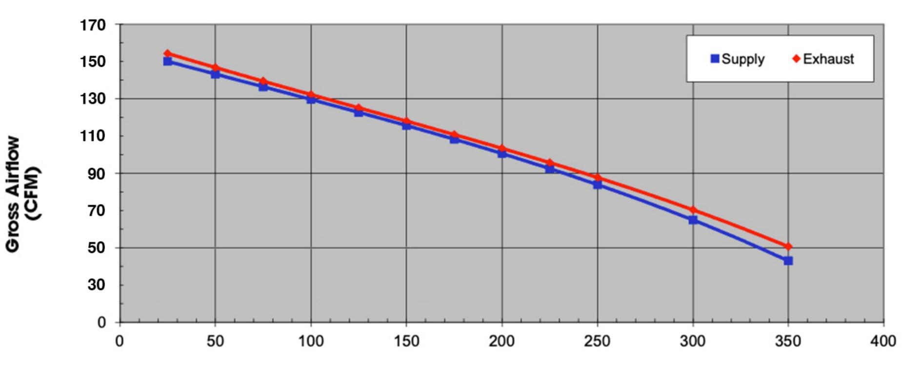
External Differential Static Pressure (Pa)
