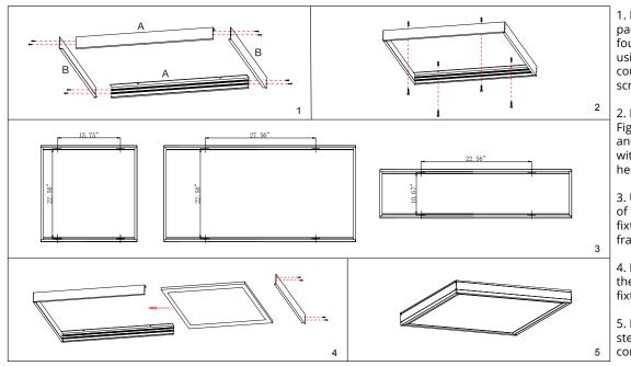
1. Remove accessories from the package carefully. Put together the four-piece surface mount kit by using the supplied ST4\*8 Cross countersunk head self tapping screws. (Fig 1)
