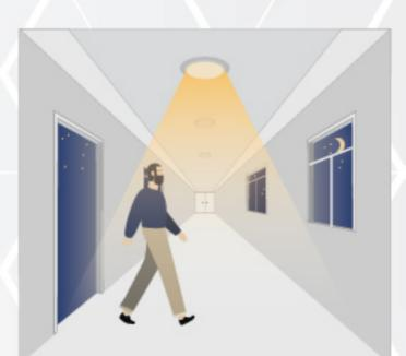
When sensor detects motion or presence it will bring the light level up to 100%.
