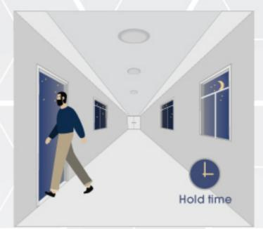
After motion is no longer detected, fixture remains at 100% for hold time.
