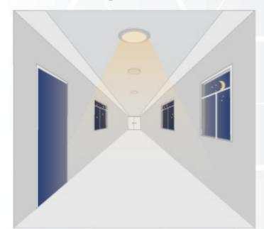
With insufficient ambient brightness, sensor turns on light and keeps it at standby dimming level even if there is no motion or persence.
