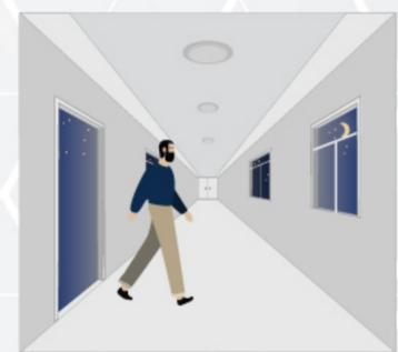
With insufficient daylight, the sensor turns light ON when motion gets detected.t
