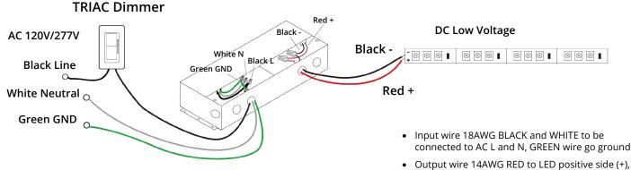
Output wire 14AWG RED to LED positive side (+), BLACK to LED negative side (-)
