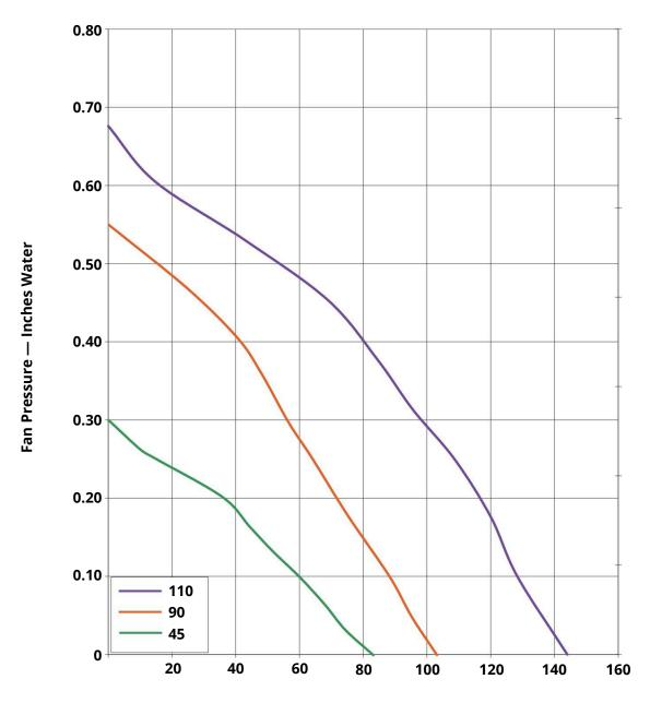
Fan Flow Rate — CFM Standard Air
