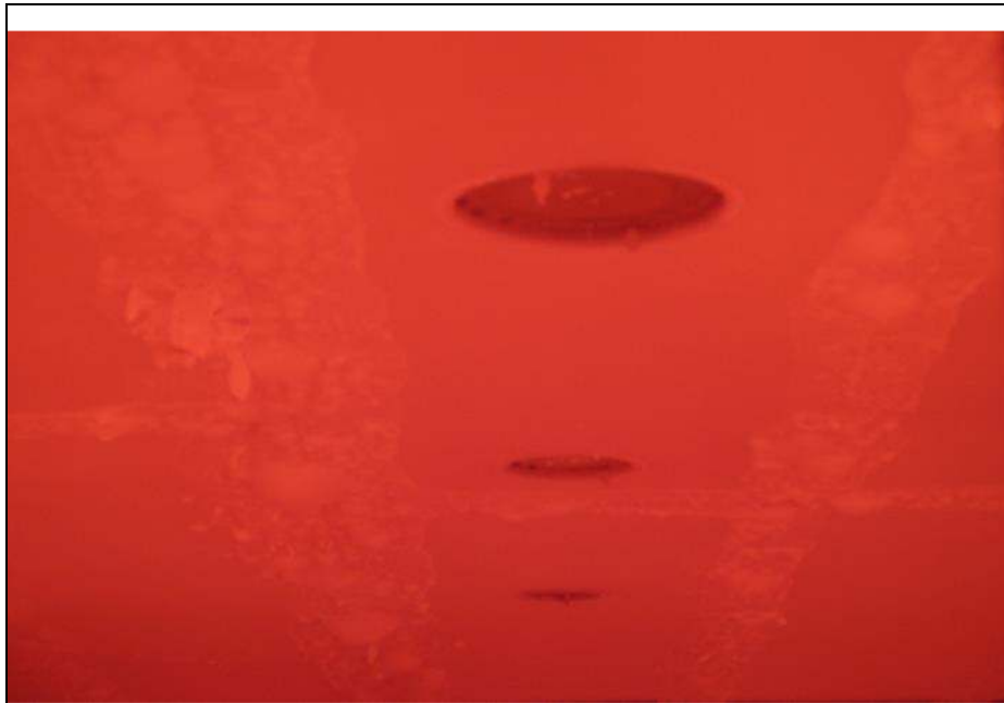
The exposed face after test duration of 120 minutes
